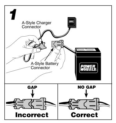
Plug the charger and battery connectors together.
